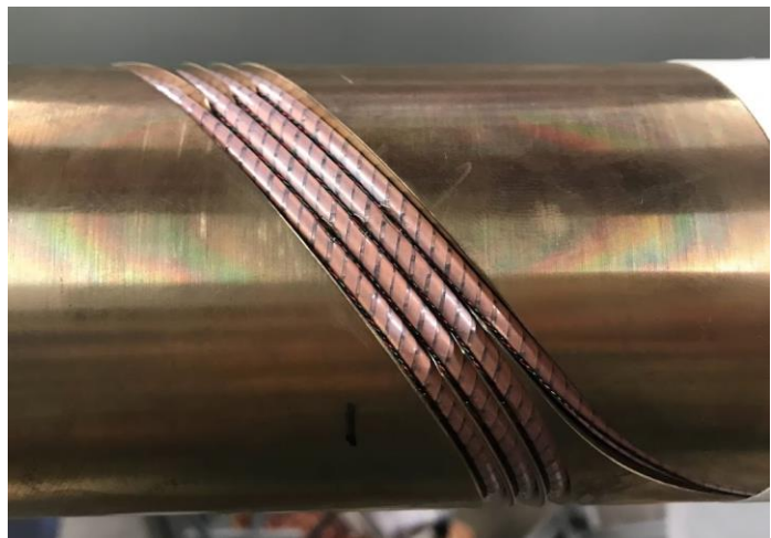
Co-wound v-tap and fiber; Maxim's new sensor in Layer 2
