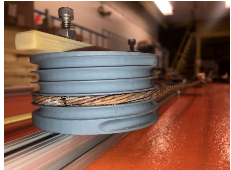
Cable bent along the groove
