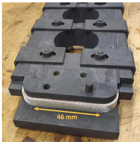
Removing the cable from the reaction sample holder.
