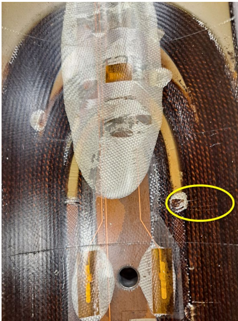
Figure 6.2: detail of coil 214 Lead End. The yellow box shows the position of “scratches” starting from the wedge to end-spacer transition
