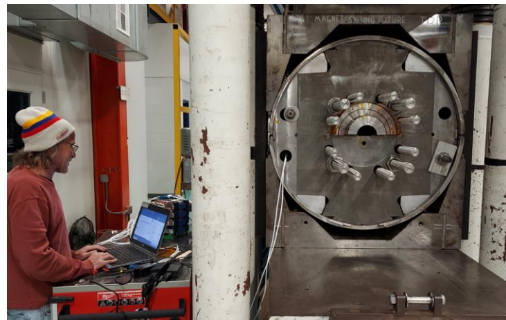
The welding contact tooling in the press
