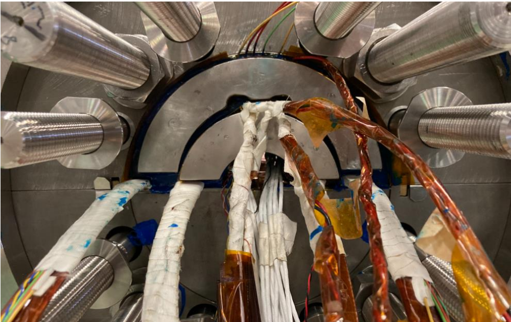
Installed pusher plates on the magnet LE
