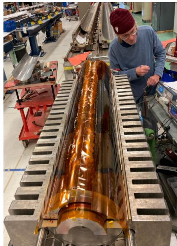
Electrical test before clamping
