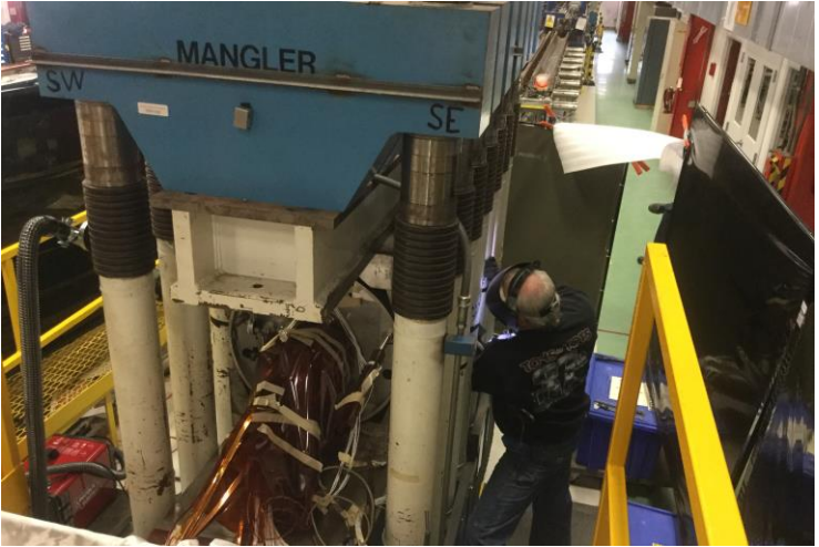
The stich welding under press load
