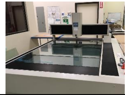
sTGC strip dimensional control with a CMM machine
