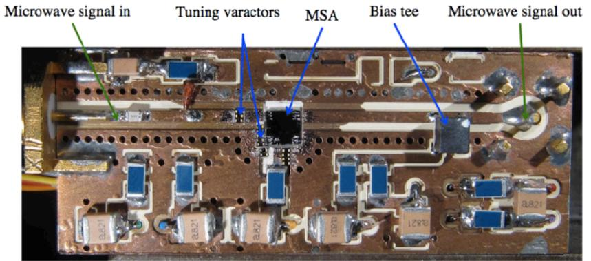
RC filtering for DC lines
