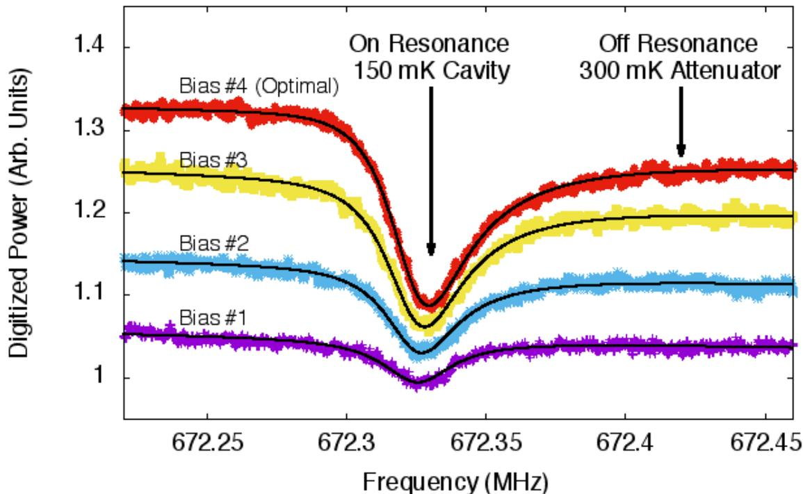
System noise temperature calibrated from difference in power between 150 mK cavity and 300 mK attenuator.
