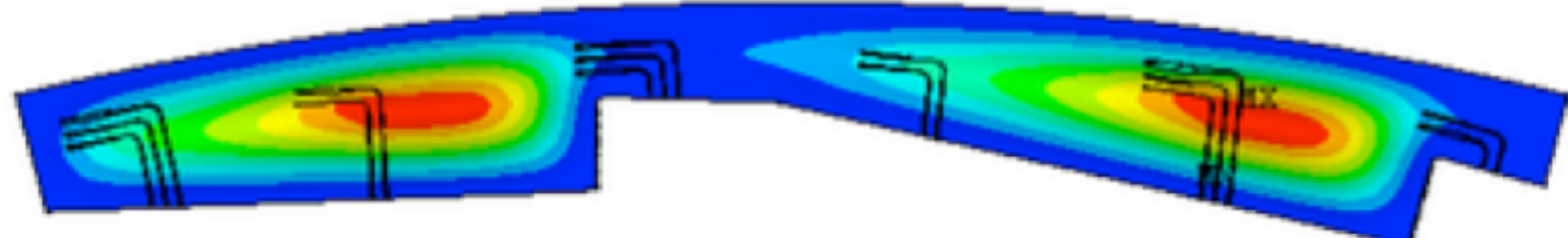
Deformation of the chamber under vacuum
