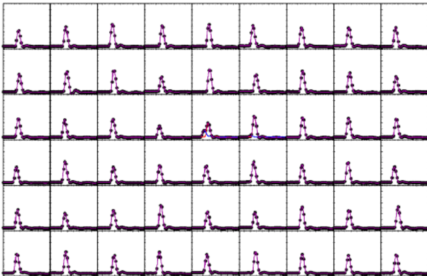
Digitized wave forms for all crystals, template fitting
