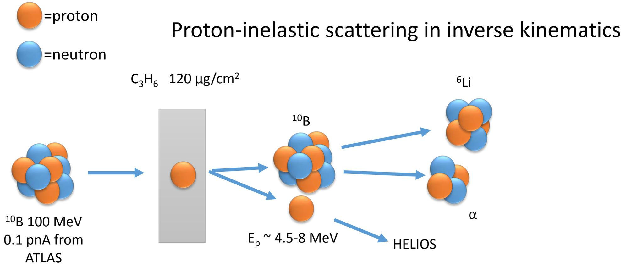
Protons detected in HELIOS; other reaction products identified in Si-Si telescopes
