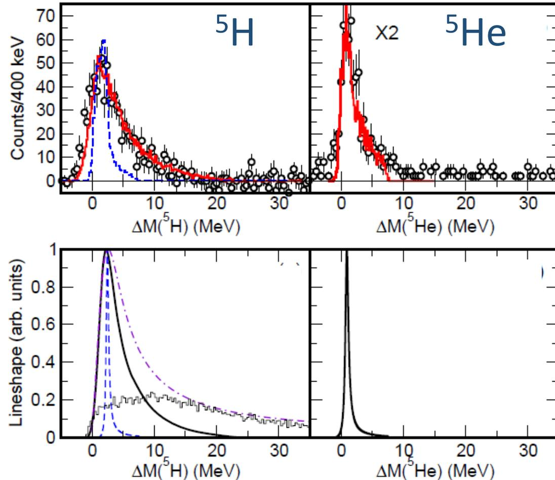
Line shapes. Thick curve: best fit; dashed-blue illustrates  ${}^5\text{H}$  resolution; Histogram: efficiency
