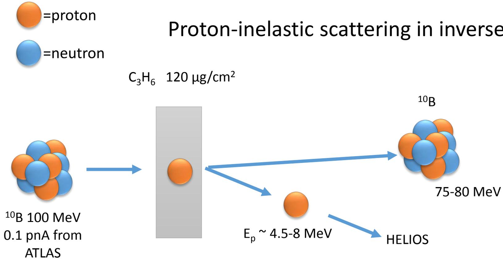
Protons detected in HELIOS; other reaction products identified in Si-Si telescopes
