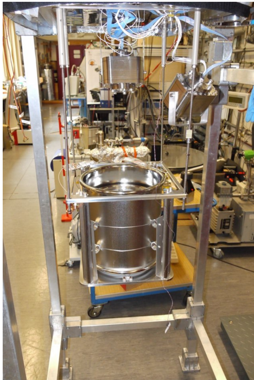
HV tests of ~30cm scale geometries
