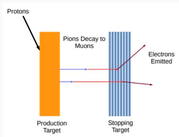
Experimental Method: Stop  $O(10^{10})$  muons per second in Al
