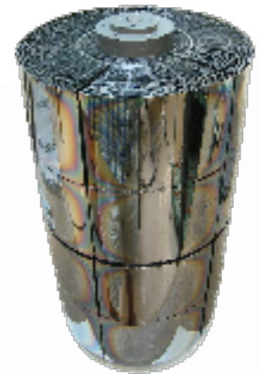
hard X-ray optics (HEFT: High-Energy Focusing Telescope)
