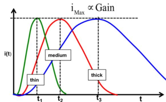
Current signals for different thicknesses
