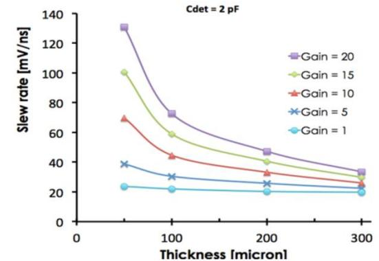
Signal slope as function of thickness.
