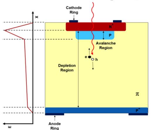
Cross section of an LGAD diode
