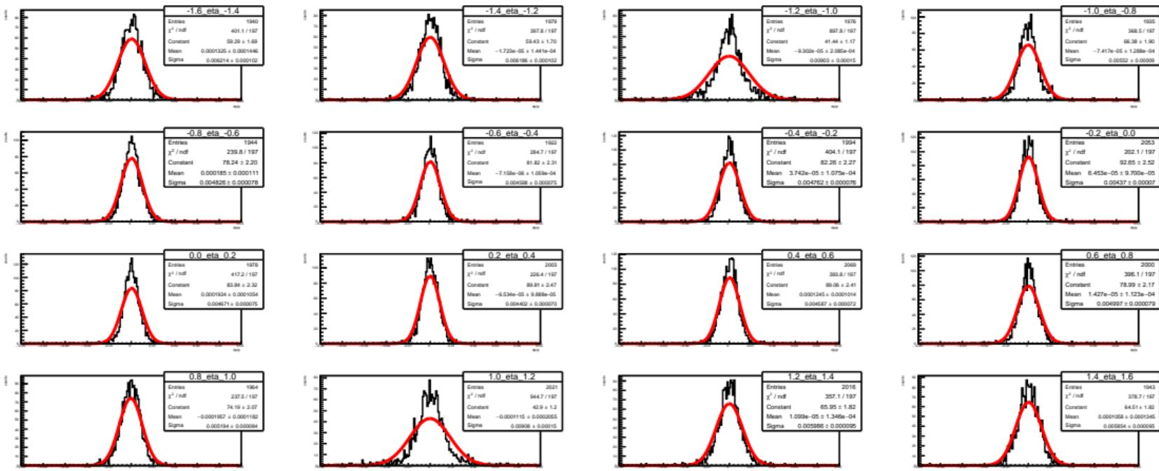
$$10 \text{ GeV: } f(x) = \frac{p_0}{\sqrt{2\pi p_2^2}} \exp\left(\left(-\frac{1}{2}\right)\left(\frac{x-p_1}{p_2}\right)^2\right) + \frac{p_3}{\sqrt{2\pi p_4^2}} \exp\left(\left(-\frac{1}{2}\right)\left(\frac{x-p_1}{p_4}\right)^2\right)$$
