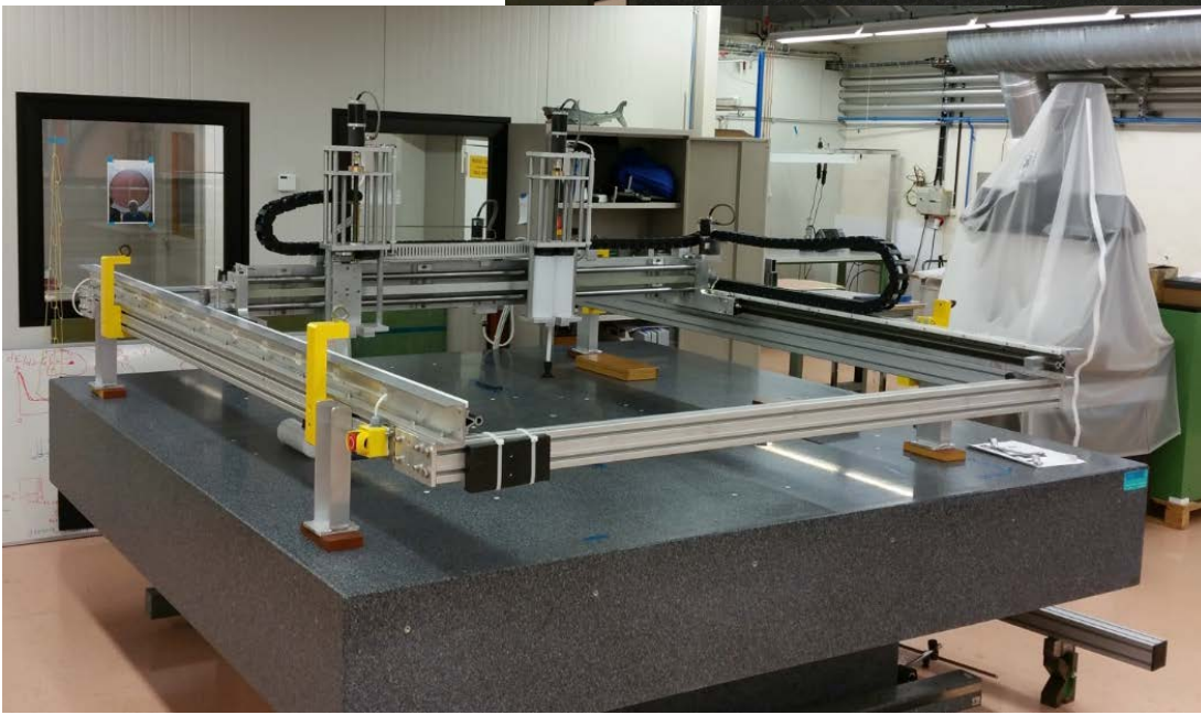
Gluing gantry machine
