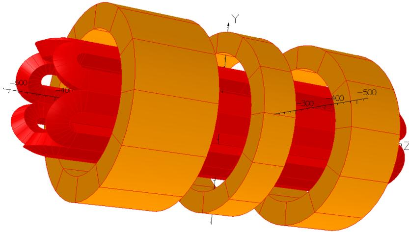
VENUS and SECRAAL-II have reached limits of NbTi superconductor in these two coil configurations
