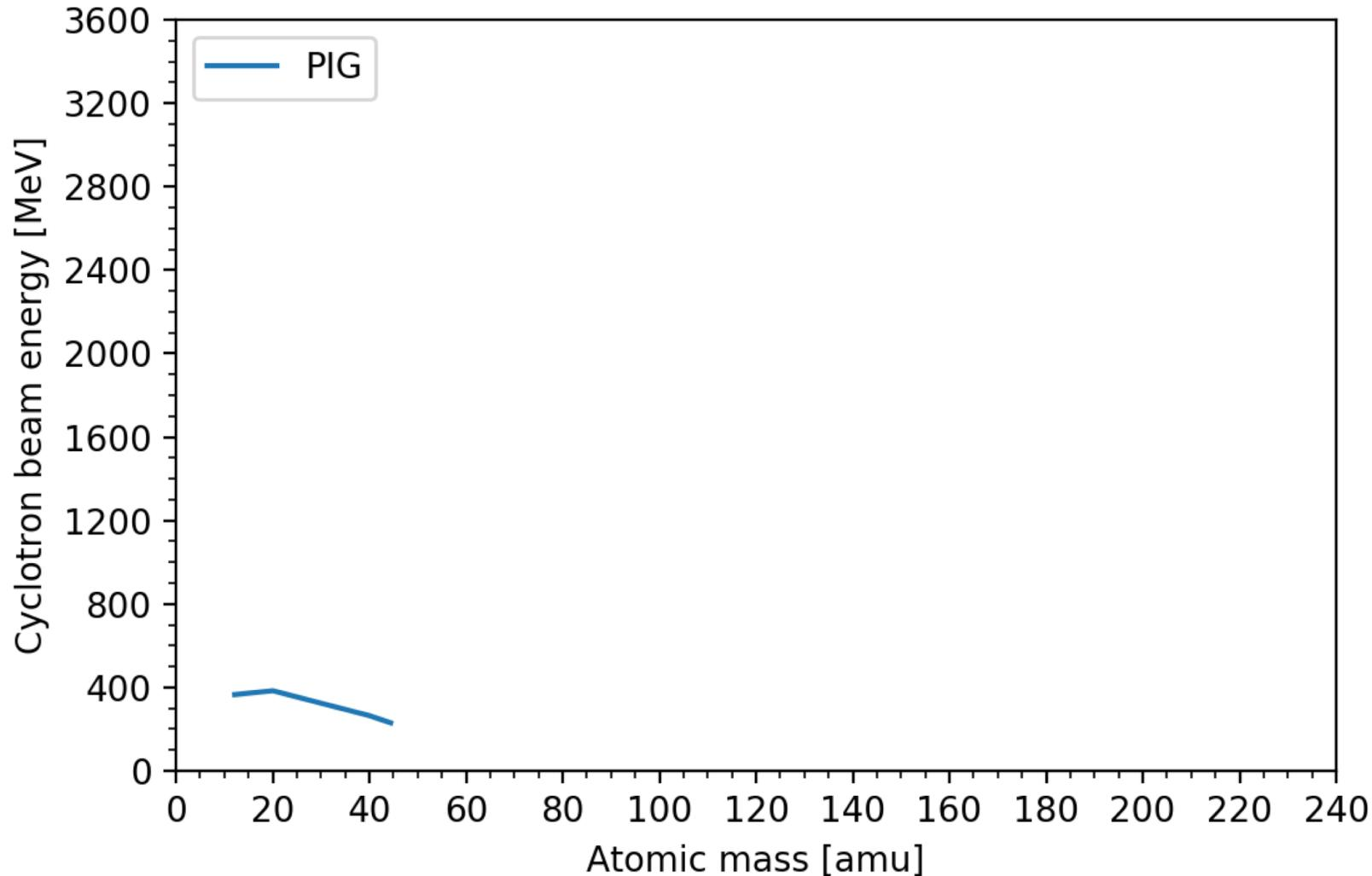
For the first 20+ years of operation, the 88" Cyclotron at LBNL used internal Penning or "PIG" sources
